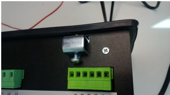
Insert the unit into cut-out in a switchboard and insert all four screw holders accordingly to their positions
