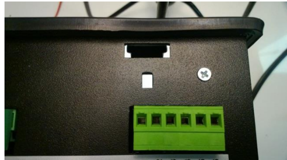
Locate four sockets for screw holders
