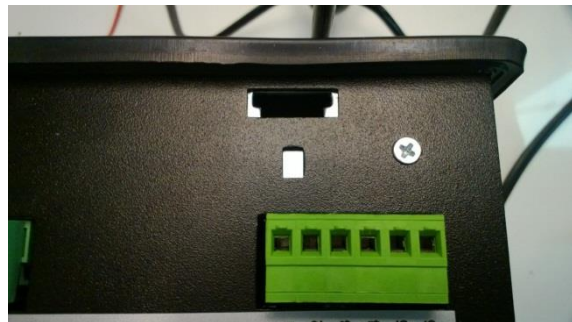
Locate four sockets for screw holders
