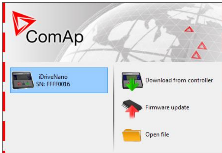
DRIVEEDIT SCREEN AFTER START – FOR CONNECTION CLICK ON DOWNLOAD FROM CONTROLLER
