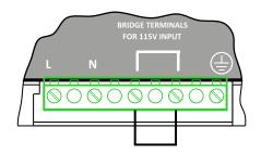
When 115  $V_{AC}$  input voltage is used bridge corresponding terminals on AC input terminal block *(see left)*.
