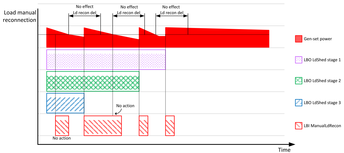
Image 5.55 Load manual reconnection
