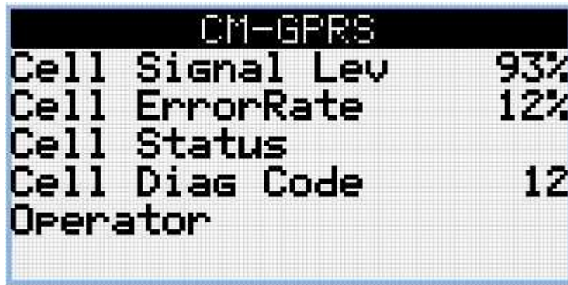
Image 10.21 Main screen of CM-GPRS module
