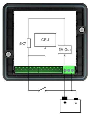
Figure 4.18 RECOMMENDED BINARY INPUTS WIRING
