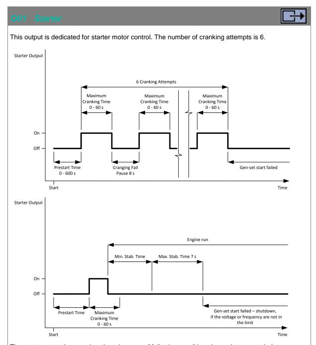
The starter output become inactive when one of following conditions is reach or exceeded.
