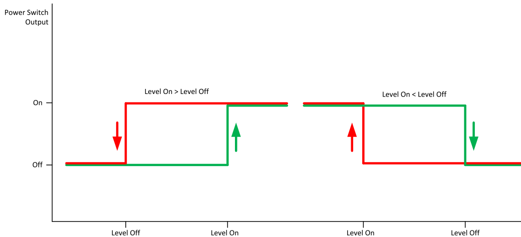
Image 9.12 Power Switch Level On > Level Off
