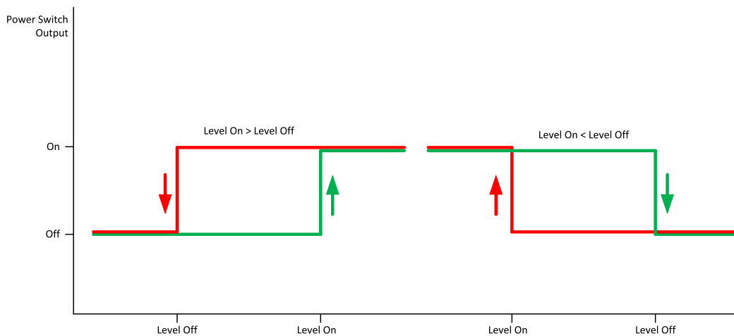
Image 9.11 Power Switch Level On < Level Off
